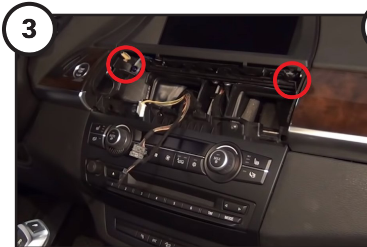
Remove the two screws securing the upper OEM display. Disconnect and remove the display.
