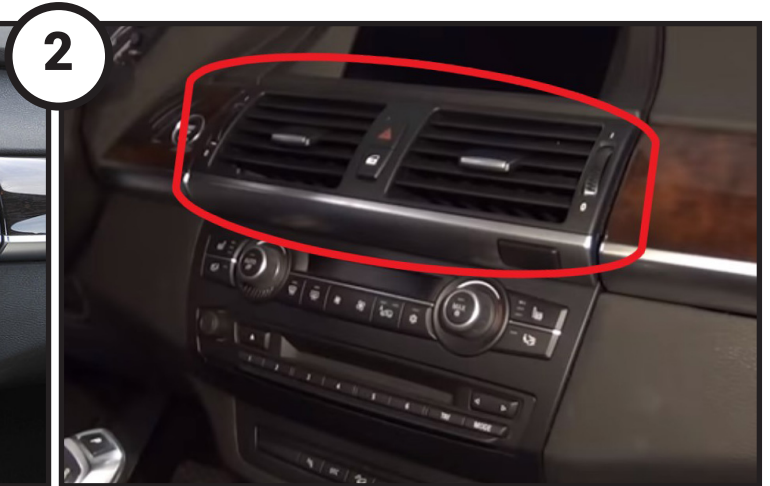
Use a panel removal tool to remove the air vents (circled).
