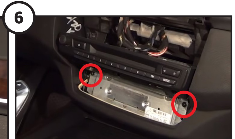
Remove the two screws securing the OEM head unit in place. Disconnect and remove the head unit.
