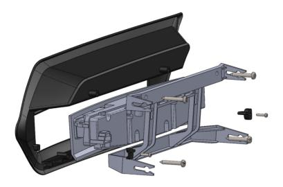
Insert the buttons into the relocation panel. Insert below the top lip and click into place. Scew the relocation bracket to the panel using the four holes on the back.
