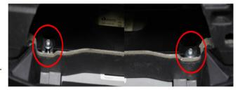
**4.** Remove the head unit and unplug all connectors attached, including the connector attached to the fascia panel of the head unit.
