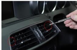
2. When removing the air vent panel, unplug the blue connector to the air vent controls.
