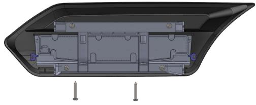
Screw the final two screws into the bottom of the bracket as circled.
