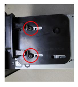
**8.** Insert the head unit and wiring assembly into the dash. The head unit is slotted into place via the guide rails as the reverse of step 3. Test the head unit for correct operation and move on to button relocation panel assembly
