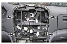
3. Unclip the front panel and remove it
