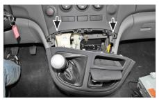
2. Unclip the gear lever box
