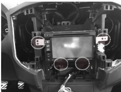
Fix the radio-frame and reassemble all the parts in the reverse order, doing all connections. Check the proper functioning of the whole system. Mount the facia plate on the dashboard.
