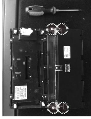
Unscrew and remove the display panel from the original plate; save the screws. Remove and save the six white clips from the original plate.
