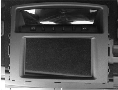
Place the white clips and the display panel, previously stored, on the supplied facia plate.
