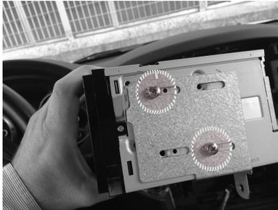
Take the left and right brackets and mount them on the AFT unit with the supplied screws. Connect all cables and, if necessary, the services bullets.
