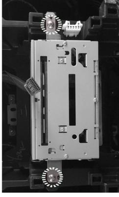
Unscrew the two screws and remove the original head unit.
