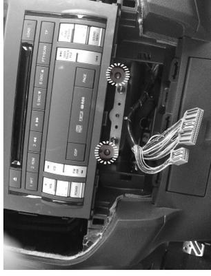
Unscrew the two screws and remove the cover panel with radio unit controls.
