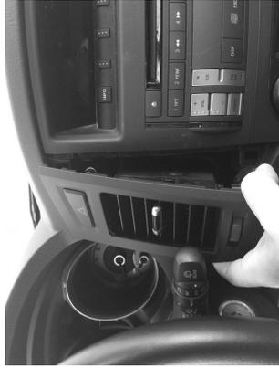
Remove the air vents and unplug the connectors.
