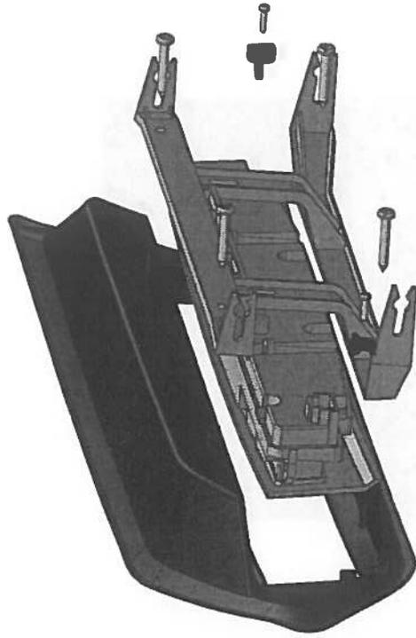
Insert the buttons into the relocation panel. Insert below the top lip and click into place. Sew the relocation bracket to the panel using the four holes on the back.
