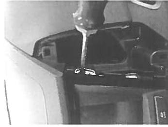
Unscrew the screws of the original radio and remove it.
