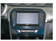
11. Connect all required circuit points. Mount Double-DIN head unit on dash board and fix it. Reinstall everything in reverse order Double-DIN Navigation
