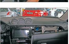
4. Suzuki Vitara dash board after removing center panel
