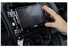
12. Once all the connections are in place, insert the new Radio carefully in the dash to avoid damage to the leads. We recommend to try the Radio is working before the screws and fascia are fitted
