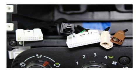
5. Connect the interface between Radio and Car Harness as shown on the images below (please note harness, USB and antenna are not included with this Facia. Process shown is for illustration only)
