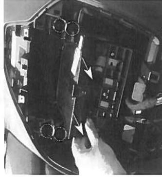
Unscrew and store the four screws and remove the plastic panel.
