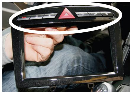
10. Mount top panel with hazard light switch to double DIN facia plate
