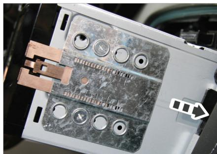
9. Attach mounting frames to double DIN head unit
