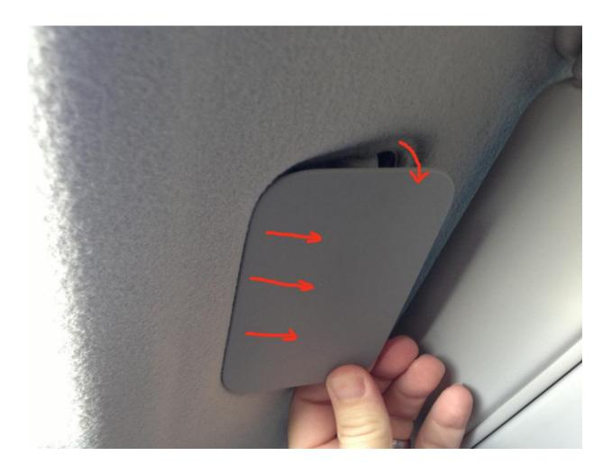
and the cover over the two screws that hold the visor on. Then I also removed the visor. Once I could see the factory microphone above the headliner, I unsnapped the factory microphone, removed the tape, and unplugged the <u>wire harness</u>.
