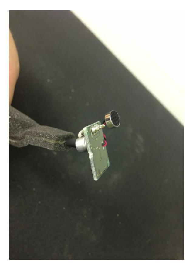
I soldered the factory microphone to the Pioneer cable, White wire to where the factory Red wire was, black to black. I used some hot glue to assure it would stay put.
