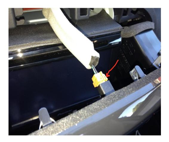
The 4 screws holding the two radio brackets can now be seen, remove the screws and then pull the radio towards you, unplug the 4 harness connectors from the rear of the stereo. Remove the brackets from the stereo using a Torx T-20 (I think). The brackets will be installed on the new stereo.
