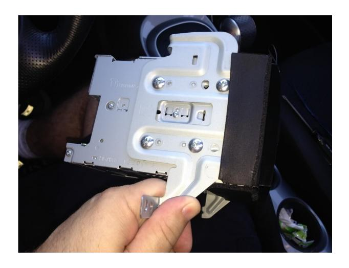
Only 2 of the connectors will be used, the largest one and the skinny <u>antenna</u> one, I wrapped the unused ones in soft foam tape to prevent any vibration.
