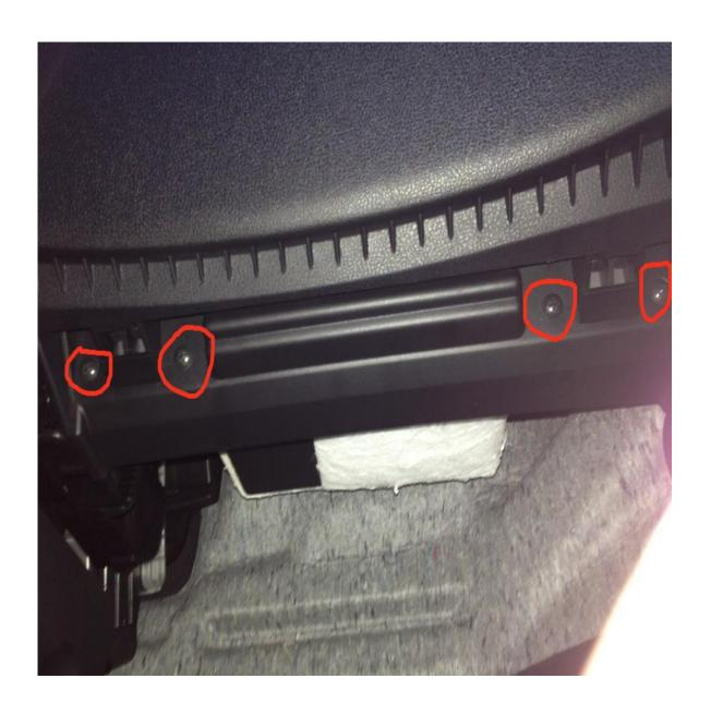
Once all the screws are out, it can be pulled towards you and slightly down with the glovebox door open just a little. There is a small harness connected to the glove box light on top, and on the right is the iPod interface jack, unplug both, if so equipped, and then move the glovebox out of your way.
