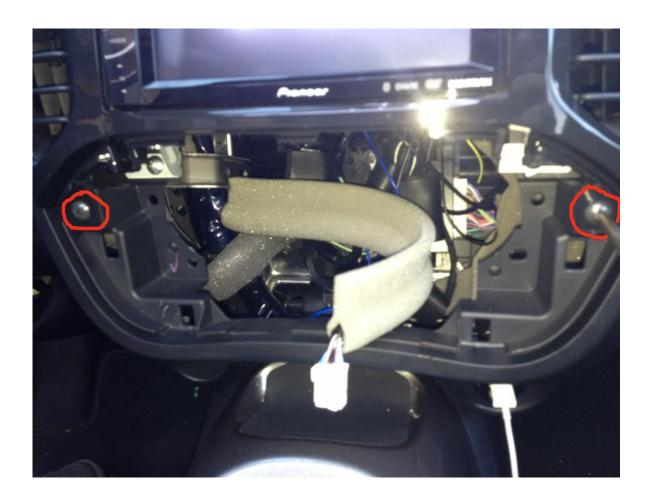
Remove the screws and then snap the bezel loose, you may have to lift the <u>window</u> wiper control shaft for it to clear. Unplug the <u>Airbag</u> warning light connector and place this bezel in a safe place also (They are easily scratched).
