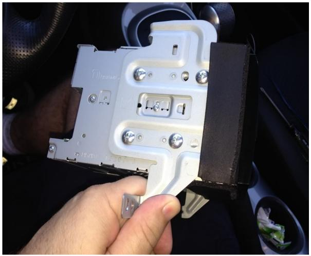
You should be able to plug in the 1/8 headphone type jack from the ASWC-1 into the the first jack on the drivers side (when the face of the unit is facing as it will installed), the tiny microphone jack is second from the drivers side, and the harness and <u>antenna</u> is on the other side.
