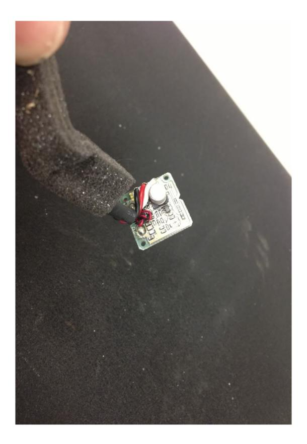
I then removed the Pioneer cable and de-soldered the Pioneer microphone. The lapel like mounting is removed by pulling the end piece off and then microphone can be pushed out the end using the wire. On the factory microphone I marked the side with the RED wire with a perminant marker and then de-soldered it from the factory wires.
