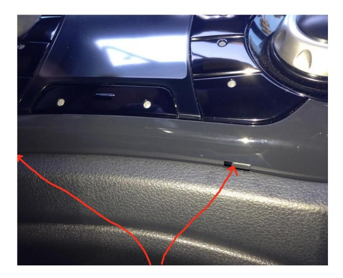
Lift up and pull it out towards you with the removal tool or screwdriver being sure the tool is well inserted behind the face to avoid it slipping out, you may need to give it a good tug to free the snaps.
