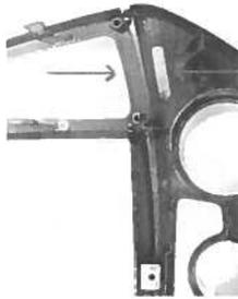
Reassemble the remaining parts on the new fascia plate and mount the radio using mounting brackets (included)
