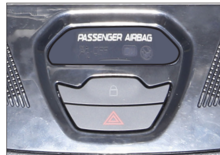
8. Mount „HAZARD LIGHT SWITCH“ and „PASSENGER AIRBAG“ display to new fascia plate
