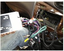
With a 29-606 and a patch lead to suit the make of head unit, connect and test the operation of the steering wheel controls.
