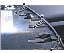
Remove air vents carefully (double clipped /see arrows) and air vent trim frames from OEM panel.
