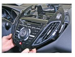
5. Unclip and remove center console
