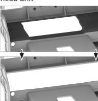
8. After cutting reinstall plastic frame into dashboard
