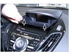
Unclip and remove panel on top of B-MAX dashboard (see arrows)
