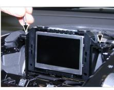
3. Remove two TX20 screws of display Remove display
