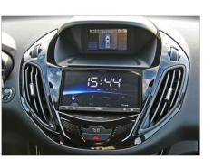
12. A new hazard light switch by Ford is required: part-no.: 1519127Attach hazard light switch to new facia plate
