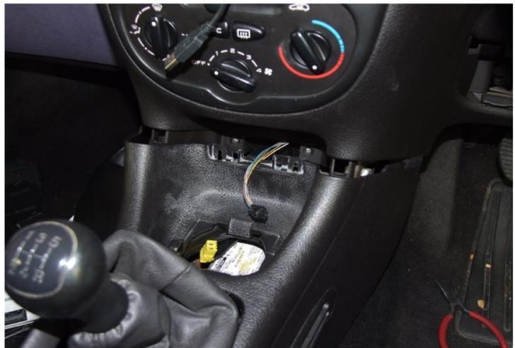
Once hazard wiring is through the gap, the centre console, ashtray light and window switch can be refitted in reverse of removal. The front screws will not be refitted. Do not fit the ashtray at this stage.
