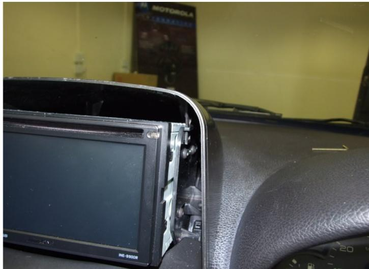
The front part of the hood has a trim which may or may not be needed depending on the stereo choice. Fitting the trim is just a case of pushing it onto the lip of the front panel taking note there is a rounded corner and a square corner
