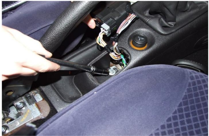
Unwrap hazard switch wiring to leave enough to allow the wire to reach the ashtray.
