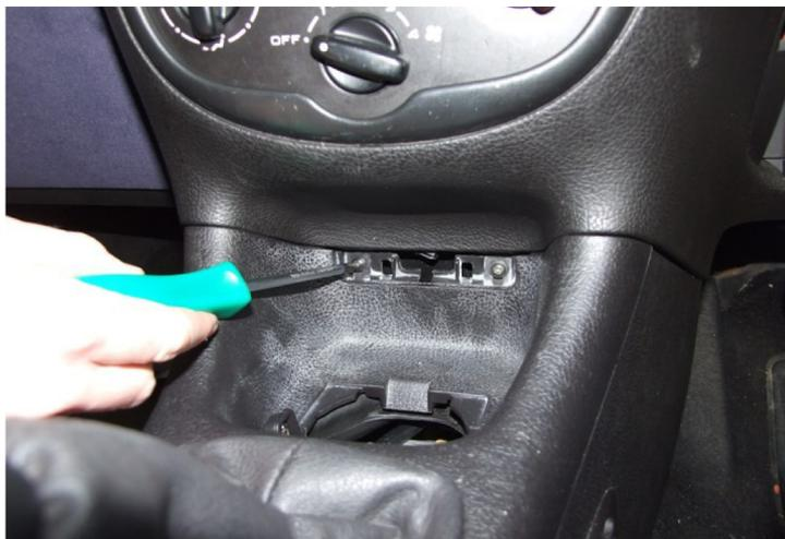
Remove window control switch panel to reveal a 10mm nut holding the centre console in place. Carefully remove the nut.
