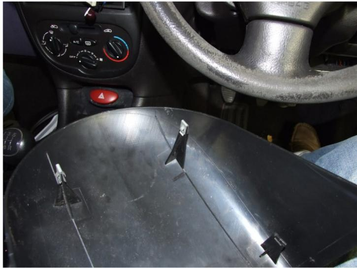
Locate the hood front clips into the stereo side brackets. Once the clips are in place, push down to clip the hood into place.
