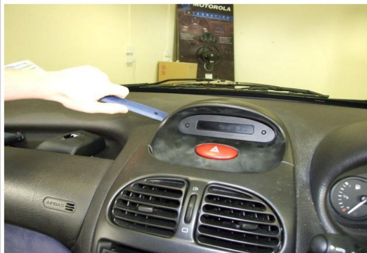
Remove screws holding display and remove display. Disconnect wiring and push wiring out the way.
