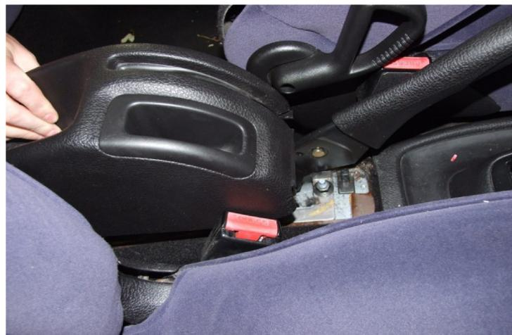
Remove the ashtray by opening and pulling upwards
