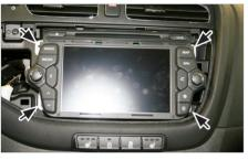
2. Remove screws of OEM head unit
