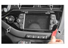
Unclip and remove OEM-panel surrounding head unit
