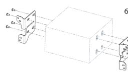
Attach mounting frames left/ right to double DIN head unit
