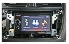
7. Place double DIN head unit Fix it with 4 screws
