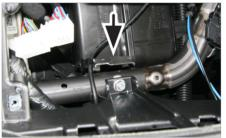
5. Bend down metal in order to clear space for double DIN head unit
