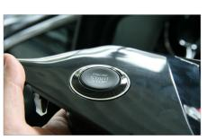
3a. Mount "Engine Start/Stop" button to new facia plate
