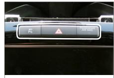
6. Remove button unit from OEM head unit
