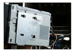
8. Attach mounting frames to double DIN head unit
