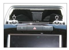
4. Remove screws of OEM head unit
