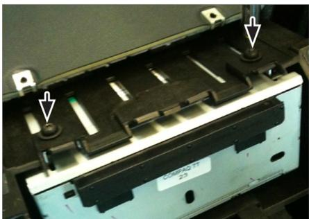
14. Remove screws of OEM Radio/CD unit
