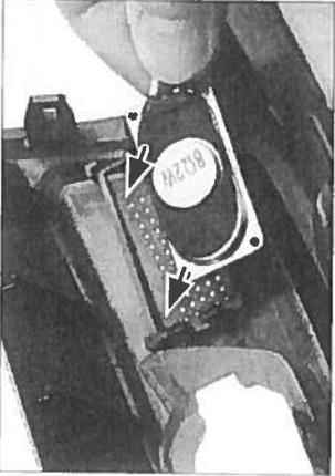
15. A spare OEM hazard light switch by Ford is required.
