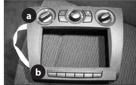
15. Attach air condition control unit (a) and switch bar (b) to replacement facia plate
