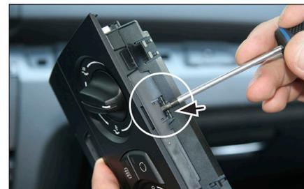
7. Unclip and remove air condition control unit
