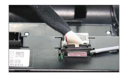
5. Remove plug attached to ribbon cable
