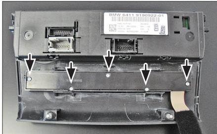
11. Remove 5 screws from switch panel ( see arrows)
