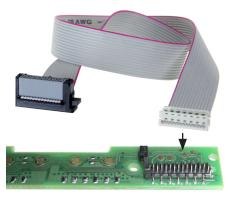
13. Attach white plug of replacement ribbon cable to PCB
