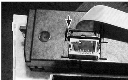
14. Attach black plug of replacement ribbon cable to air condition control unit
