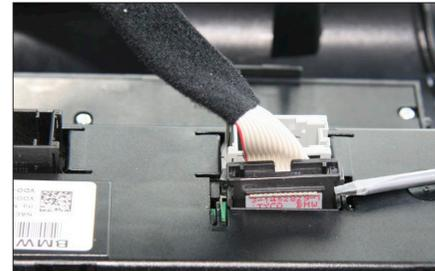
5. Remove plug attached to ribbon cable
