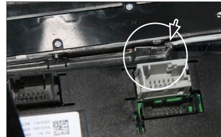
6. Unclip and remove switch panel below air condition control unit
