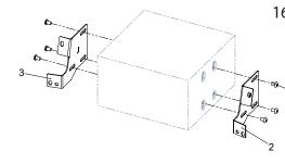
16. Attach mounting brackets to double DIN navigation
