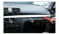
Unclip middle panel and remove it carefully
