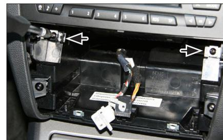
8. Remove screws below OEM head unit (see arrows)
