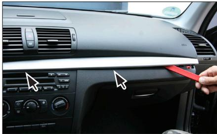
2. Unclip middle panel and remove it carefully
