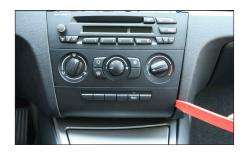
B. Unclip air condition control unit
