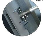
3. Remove screws below OEM head unit (see arrows)
