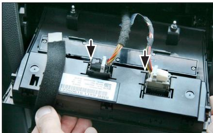
4. Pull out air condition control unit carefully
