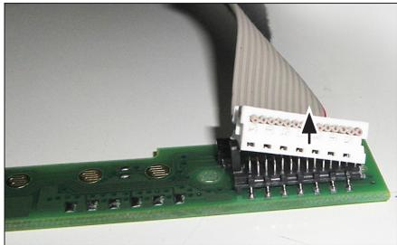
12. Remove plug attached to ribbon cable from PCB
