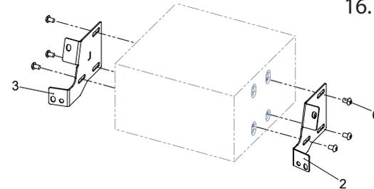
16. Attach mounting brackets to double DIN navigation
