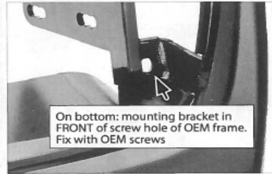
On bottom: mounting bracket in FRONT of screw hole of OEM frame. Fix with OEM screws
