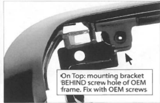
On Top: mounting bracket BEHIND screw hole of OEM frame. Fix with OEM screws
