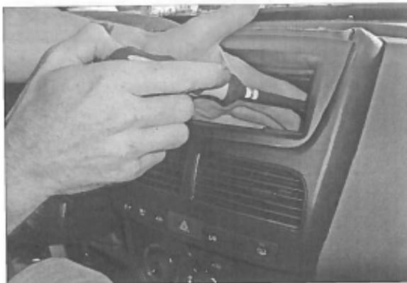
2. Remove 2 screws (left and right)
