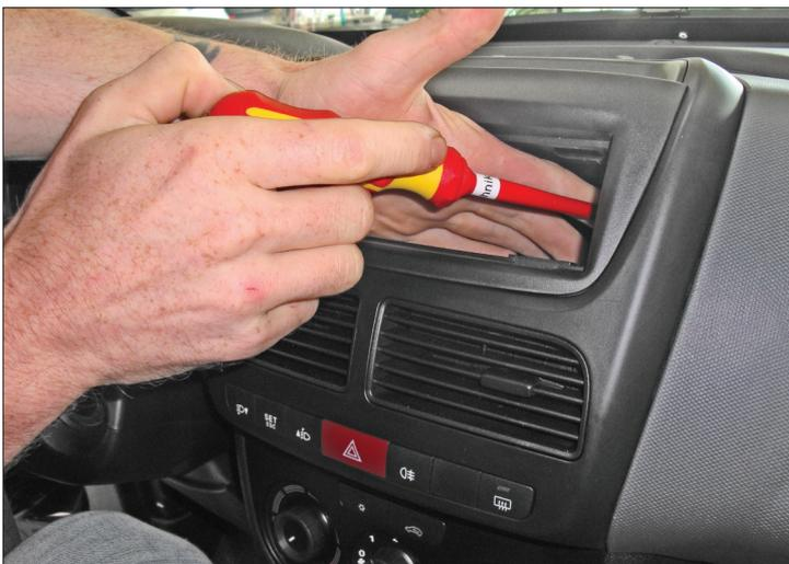
2. Remove 2 screws (left and right)
