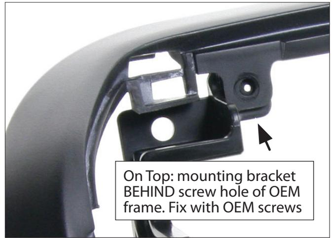
On Top: mounting bracket **BEHIND** screw hole of OEM frame. Fix with OEM screws
