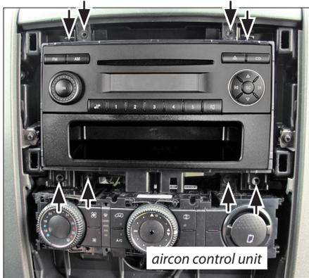
2. Remove the OEM radio and the aircon control unit.
