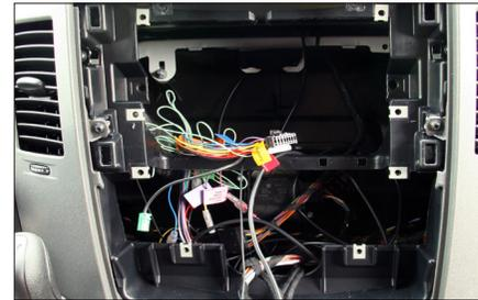
3. Dashboard with removed OEM radio and aircon control unit.
