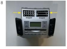
Rem ove the air shafts from the original radio and replace them in the OEM replacem ent panel.
