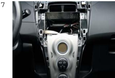
7 Place the metal bracket into the dashboard between the OEM brackets.
