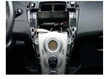
Place the m etal bracket into the dashboard between the m etalOEM brackets.
