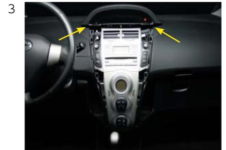
3 Lift up the panel above the air shafts at the location of the arrows by using a plastic wedge.
