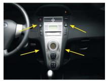
Rem ove the dashboardpanels around the radio at the location of the armows.
