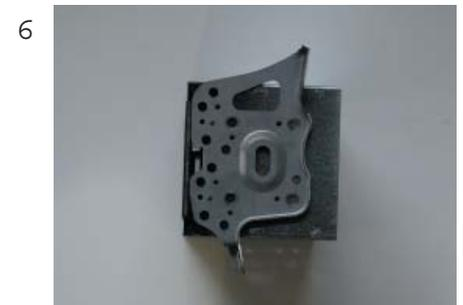
6 Place the OEM radio brackets on the metal bracket of the new headunit. This will fit in the holes of the metal bracket (if needed mount it with screws).
