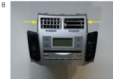
8 Remove the air shafts from the original radio and replace them in the OEM replacement panel.
