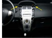
Lift up the panelabove the air shafts at the location of the arrows by using a plastic wedge.
