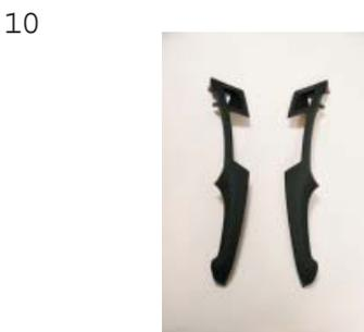
10 You need the OEM side dashboard panels for placing the new headunit.
