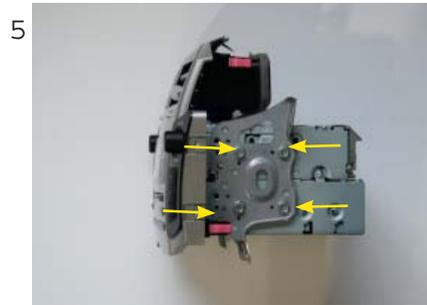
5 Remove the original OEM metal brackets from the radio. This is tightened by eight screws.
