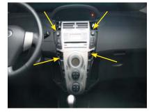
Rem ove the OEM radio at the location of the arrows. The radio is tighten by four screws.
