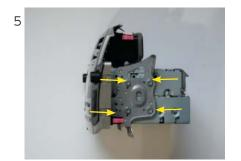
Rem ove the originalOEM m etalbrackets from the radio. This is tighten by eight screws.
