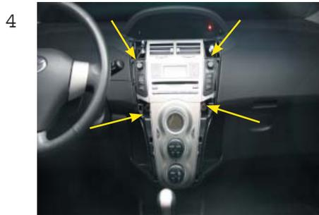
4 Remove the OEM radio at the location of the arrows. The radio is tightened by four screws.
