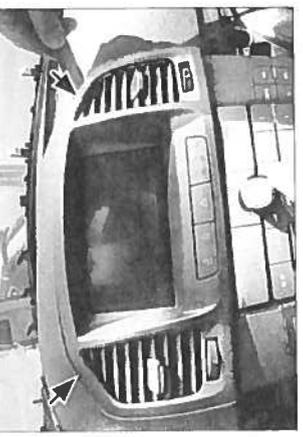
5. Unclip and remove OEM display
