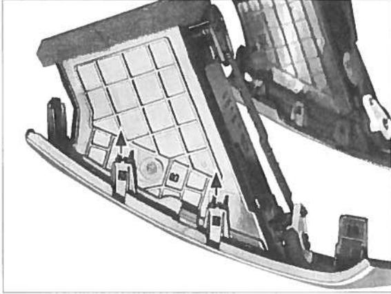
17. Remove the air vents of the original panel (left and right)
