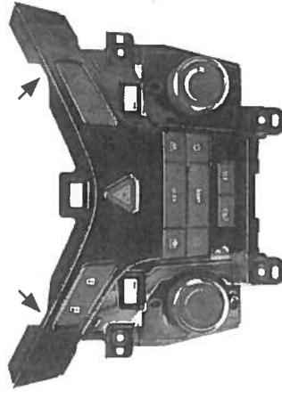
11. After cutting out of edges the OEM panel should look like this (see sample picture)
