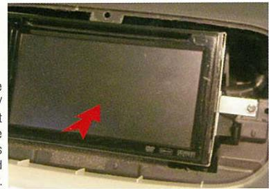
**6.** Insert the Radio / DVD / Navigation unit into the cage until the springs click and engage fully.
