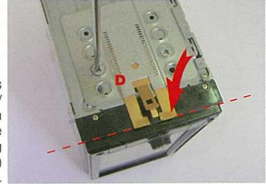
**5.** Apply the springs (D) to the Radio / DVD / Navigation unit using the mounting hardware (D) as necessary.
