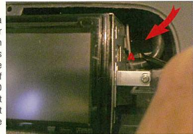
**7.** Using a screwdriver, or similar, push the paddles (A) against the sides of the Radio / DVD / Navigation unit to ensure correct airflow from the ventilation ducts.
