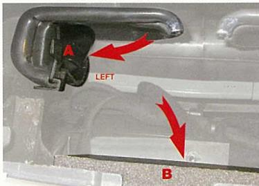
**3.** Insert the paddles (A) into the cut ducts, using the "U" section to guide the correct position. Remove backing paper and the stick the foam block (B) in central position as shown.
