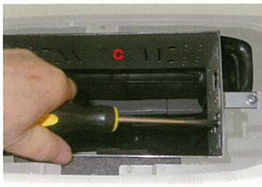
**4.** Locate the cage (C) in position, ensuring correct alignment to the foam block and screw, as shown.
