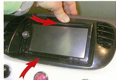
**8.** Carefully apply the Housing / Panel (E). First locate the top clips and then the lower section.
