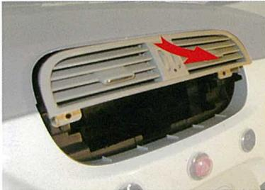
**1.** Remove the original radio and air-vent cover.
