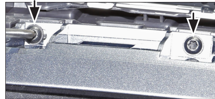
4. Remove OEM head unit by pulling it towards your direction
