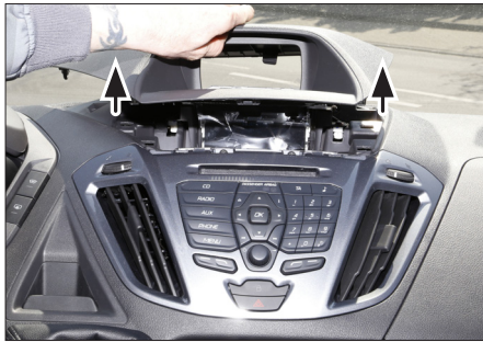
2. Unclip and remove top cover (see arrows)
