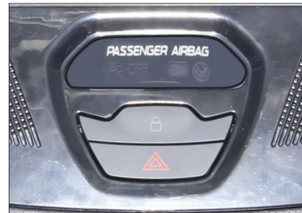
8. Mount „HAZARD LIGHT SWITCH“ and „PASSENGER AIRBAG“ display to new facia plate
