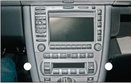
1. Remove 2 Torx (TX25) screws (1 on each side) left and right, located at the front end of the centre tunnel.
