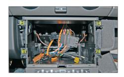
Loose one screw (head 7 mm), 4. located at the right side of the head unit.
