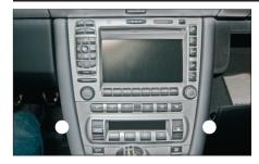
Remove 2 Torx (TX25) screws 1. (1 on each side) left and right, located at the front end of the centre tunnel.
