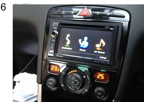
Fit the head unit into the cage, then fit the replacement panels.
