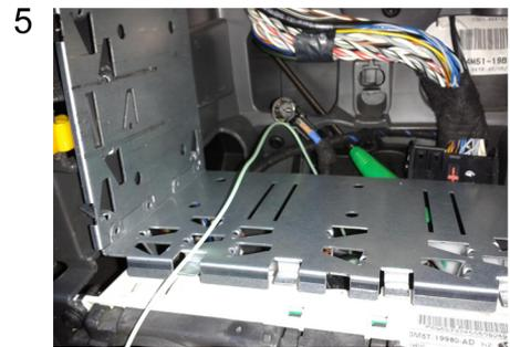
Push in the metal clip to secure the cage into place.
