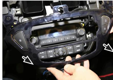
6. Remove OEM cover (unplug all connectors carefully)
