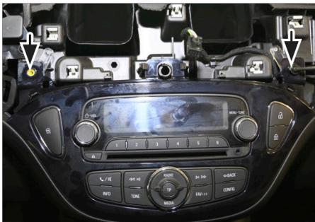
4. Remove 2 screws of head unit cover
