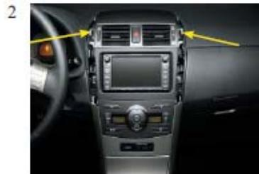
Remove the top air shaft by pulling it forwards.
