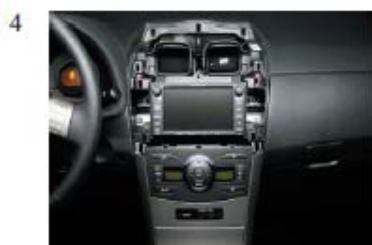
Remove the orginal radio this is tigten by four screws.
