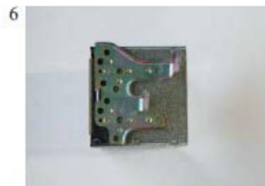
Place the OEM radio brackets on the metal bracket for the new headunit. This will fit in the holes of the metal bracket(if needed mount it with screws).
