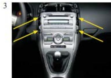
Remove the original radio at the location of the arrows this is tighten by four screws.
