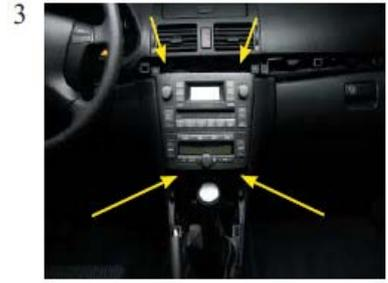
3 Remove the original radio at the location of the arrows. The radio is tighten by four screws.
