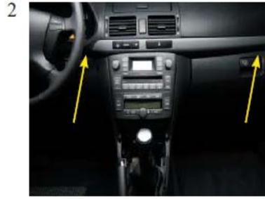
2 Remove the frame above the radio by using a plastic wedge at the location of the arrows.
