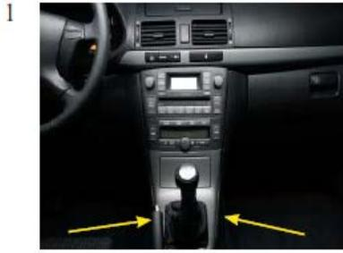
1 Remove the dashboardpanels around the radio at the location of the arrows.
