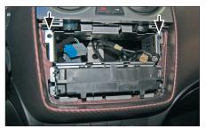
Remove the original metal holder inside the the dashboard, which is fixed by 2 screws (see arrows)
