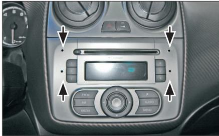
1. Insert special radio release keys in the holes of the OEM Radio
