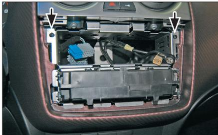
3. Remove the original metal holder inside the dashboard, which is fixed by 2 screws (see arrows)
