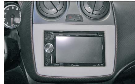
5. Push the Metal Frame into the fascia plate, place both into the dashboard.
