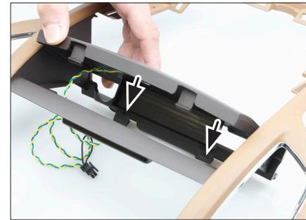
11. Clip rear side of blanking cover into OEM panel
