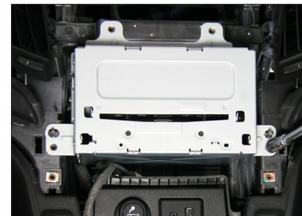
8. Remove screws of OEM head unit
