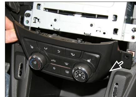
7. Remove screws of air condition control unit
