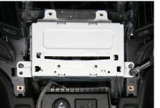
8. Remove screws of OEM head unit
