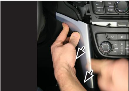
4. Unclip and remove left decor panel
