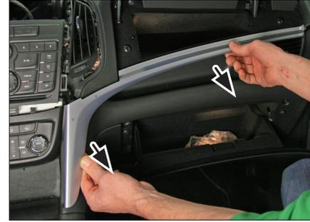
5. Unclip and remove right panel
