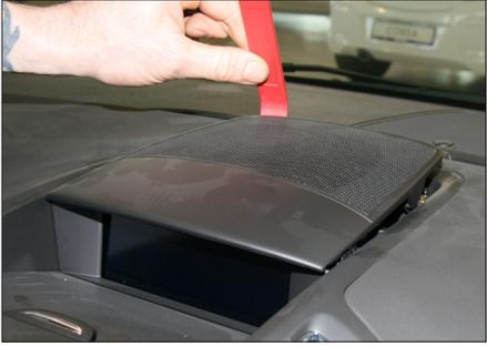
1. Unclip and remove top panel
