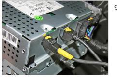
Unplug all cables of OEM head unit - and remove it
