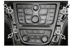
5. Remove screws of OEM head unit
