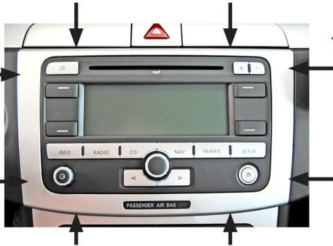
1. Remove the original trim frame, surrounding the radio (fixed by clips).
