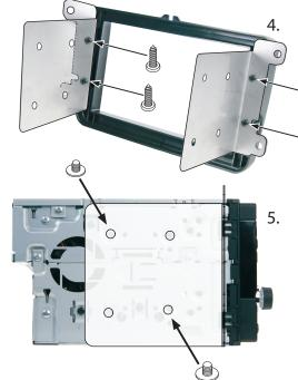
Mount both metal brackets at the facia plate as shown in the sample picture on the left.
