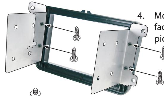
4. Mount both metal brackets at the fascia plate as shown in the sample picture on the left.
