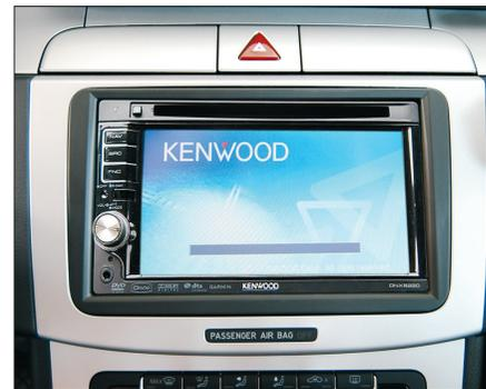
6. Connect all wires and fix the double DIN head unit with the original Torx (TX20) screws (which have been removed in step 2)
