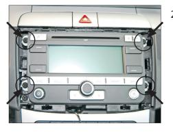
Remove the 4 Torx (TX20) screws (These screws will be used again later).
