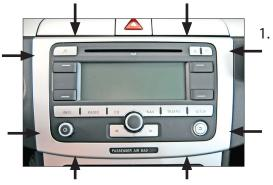
Remove the original trim frame, surrounding the radio (fixed by clips).
