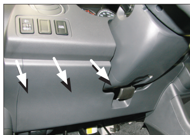
Remove dashboard cover under the steering wheel by pulling towards seat (see arrows).
