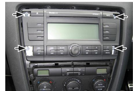
2. Remove 4 screws fixing the OEM head unit. Remove OEM head unit.
