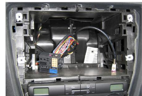
3. Place mounting frame on the dashboard and fix it with the original screws.
