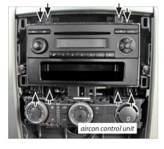
Remove the OEM radio and the aircon control unit.
