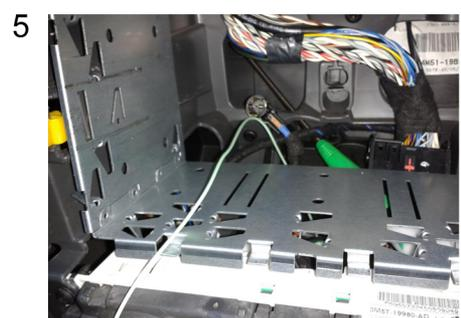
Push in the metal clip to secure the cage into place.
