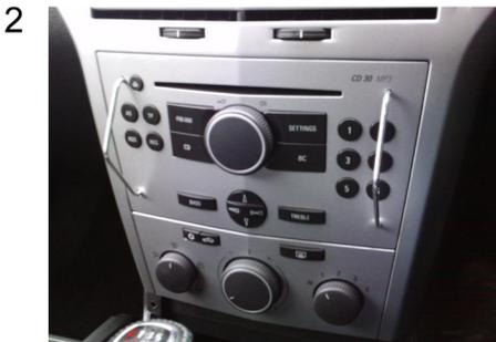
Remove the original radio using Ford radio release keys.
