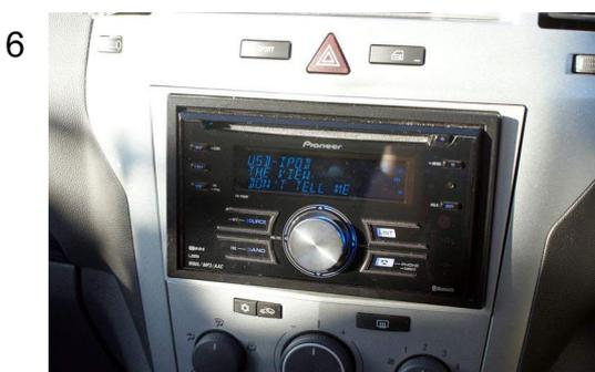
Fit the head unit into the cage, then fit the replacement panels.
