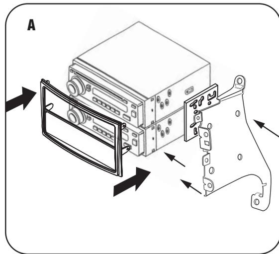
**3** Place one of the ISO spacer brackets and the left factory mounting bracket (Removed from radio during disassembly) on the left side of the ISO units. (The spacer bracket should be between the ISO units and the factory bracket.) Align the pins on the trim-plate with the holes on the factory bracket and mount the factory bracket to the ISO units using screws supplied with the radio. (Figure A)
