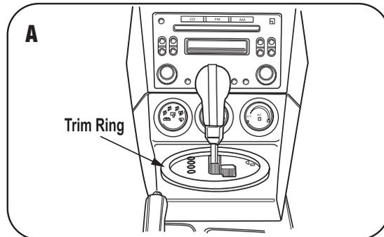
For vehicles with manual transmission, Unscrew and remove shifter knob. (Figure A)
