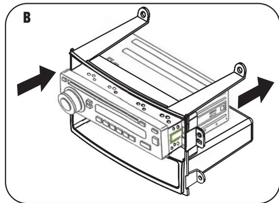
**4** Attach the radio / housing assembly to the radio trim panel using the factory screws removed during disassembly. (Figure C)
