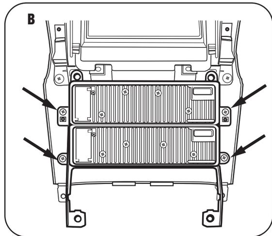
**4** Attach the assembled units and brackets to the radio trim panel using the factory screws removed during disassembly. (Figure B)
