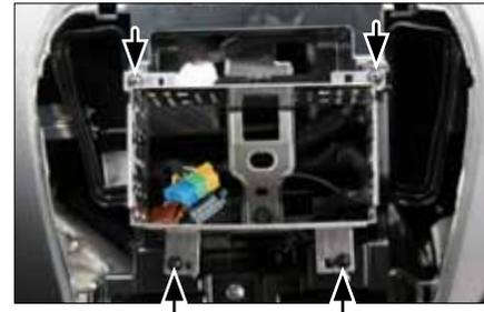
5. Place metal frame and fix it with original screws (see arrows)
