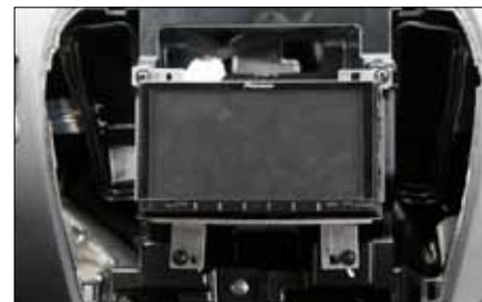
6. Push double DIN head unit into metal frame until it snaps in
