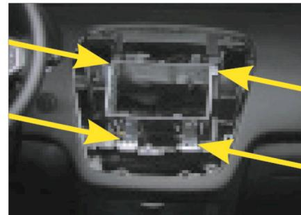
4. Place the Double DIN metal frame on the dash board and fix it with the 4 original screws.
