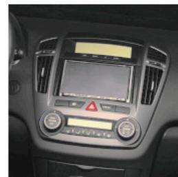
5. Connect all required circuit points to the head unit and push it into the metal frame until it snaps in. Place the fascia plate.
