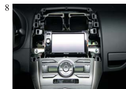
Place the new headunit
