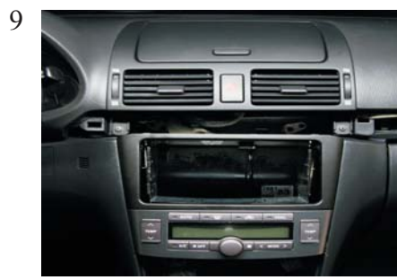
Place the OEM replacement panel with the climate control unit and the metal bracket into the dashboard.
