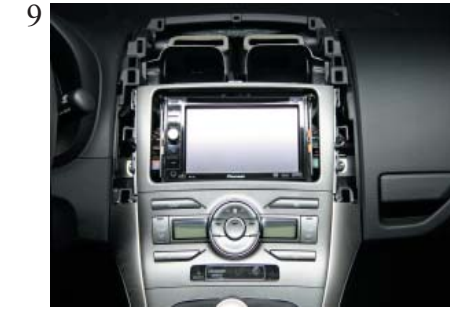
Place the OEM replacement panel.
