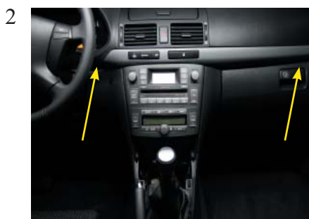
2 Remove the frame above the radio by using a plastic wedge at the location of the arrows.
