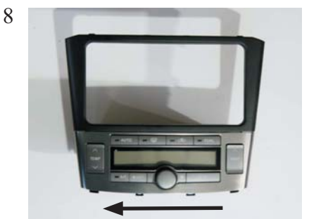
Place the OEM replacement panel on the climate control unit by sliding it to the left .
