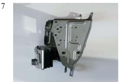
Place the new metal bracket and the climate control unit between the OEM radio brackets. Tighten the climate control with the four original screws.
