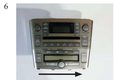
Remove the original radio from the climate control. Slide the climate control unit to the right.
