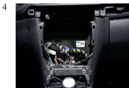
1 Remove the dashboardpanels around the radio at the location of the arrows.
