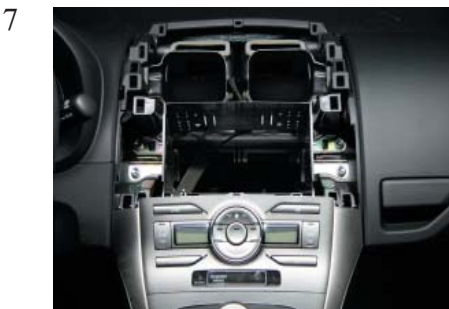
Place the metal bracket into the dashboard between the metal OEM brackets.
