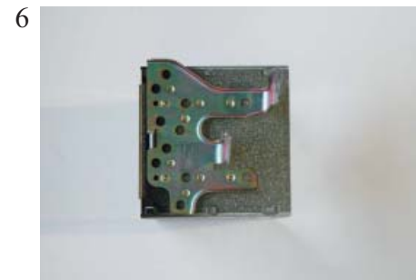
Place the OEM radio brackets on the metal bracket for the new headunit. This will fit in the holes of the metal bracket(if needed mount it with screws).
