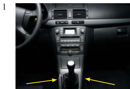
1 Remove the dashboardpanels around the radio at the location of the arrows.
