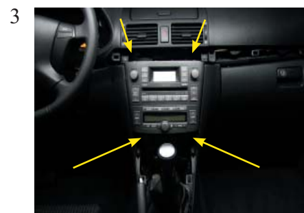
3 Remove the original radio at the location of the arrows. The radio is tighten by four screws.
