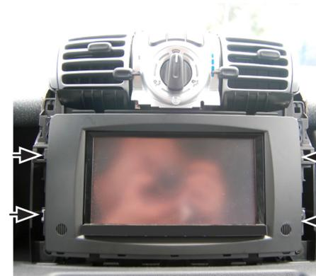
5. Push the Double DIN head unit into the metal frame, push both into the mounting frame and press the facia plate onto the mounting frame, until it snaps in.
