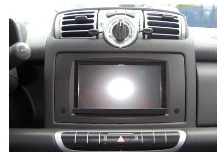
Fix the Double DIN head unit with the 4 original screws (see arrows)
