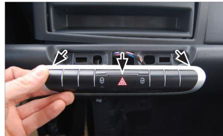
2. Remove the switch unit (fixed by clamps) by pulling it towards you
