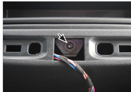
3. Remove the TORX TX25 screw holding the surrounding frame (see arrow)
