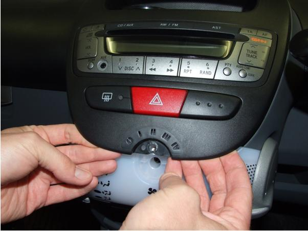
3. Disconnect the connectors from the back of the head unit.
