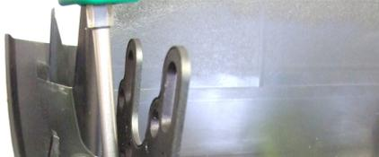
9. Take the aftermarket head unit and line it up with the holes as shown. The head unit is offered to the fascia plate from the rear.
