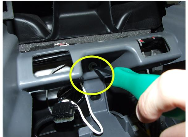
6. Cut and remove the plastic housing along the 3 lines.
