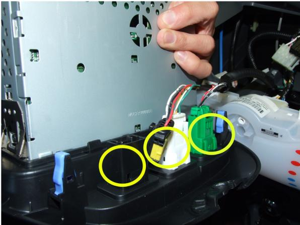
5. Unscrew the centre screw from the plastic housing at the rear of the aperture (circled).
