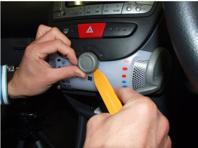
2. Remove the screw which is behind the fan control button.
