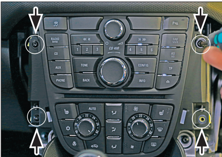
3. Remove 4 screws of OEM front panel (see arrows)
