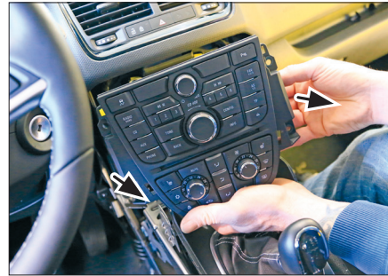
6. Pull front panel carefully into your direction in order to unplug all connectors and cables.
