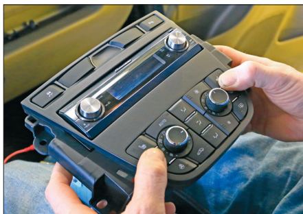
11. Mount switches and control unit to facia plate
